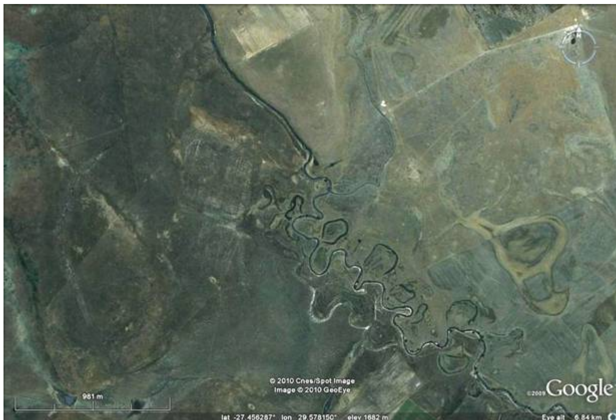
Figure 6.2 The transition from sandstones (bottom right) to dolerites (top left) causes an abrupt change in morphology of the Klip River. The wide, meandering floodplain reaches form in the sandstone zones whereas linear, confined river reaches develop within the dolerite zones
