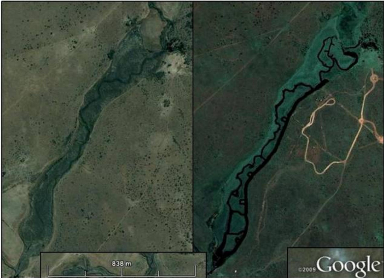
Figure 5.7 Excavation of a peat wetland above Klerkskraal Dam in the Mooi river catchment. The naturally weakly channelled wetland (left) has had channels dug into it for recreational use (right). This raises the risk of desiccation of the wetland through increased drainage, and in wetlands where heavy metals are immobilised in the anaerobic sediments, this can cause remobilisation of these toxic metals
