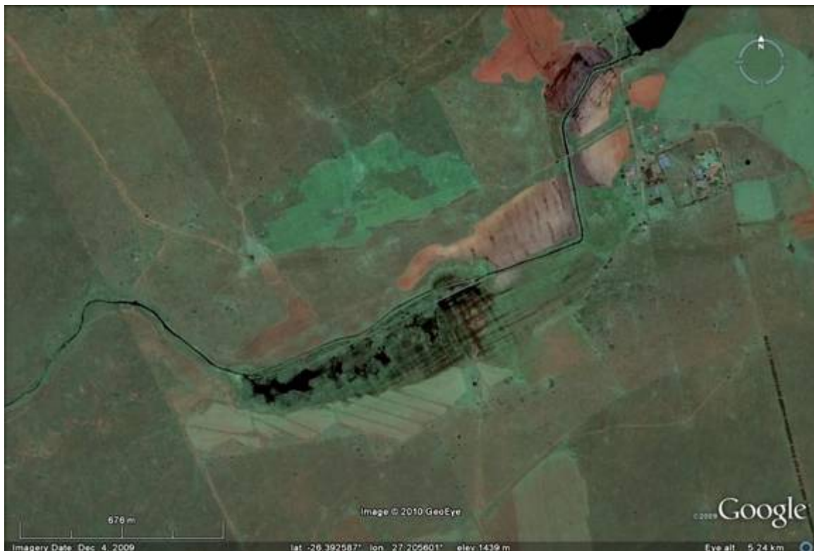
Figure 5.6 Channelised section of a wetland. Inundation and saturation of the adjacent wetland areas is likely to have reduced as a result of the channelization
